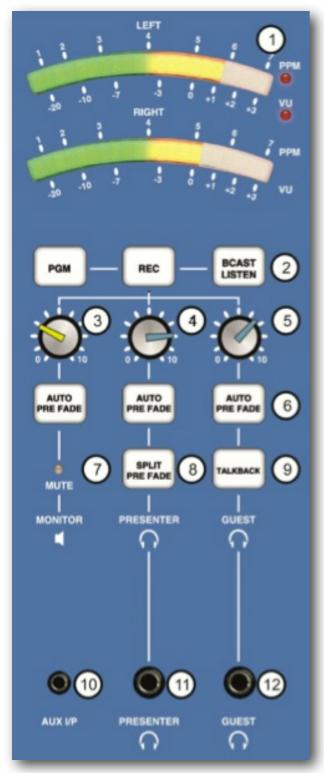
(2) - PGM / REC / BCAST LISTEN Butons: These buttons are used to select the output bus that you want the LED Meter to display (see above) plus is sent to the studio MONITORS (speakers) and PRESENTER & GUEST HEADPHONE. To switch to PGM, REC or BCAST Listen, just press the button. The bus that the LED Meter is currently displaying is indicated by the button being illuminated. One of these options will be selected at all times.
