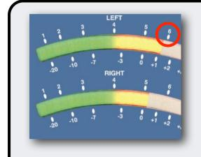
Make sure PGM is selected below the level meters and take level from your microphone - you are aiming for a maximum of 6 on the level meter.
