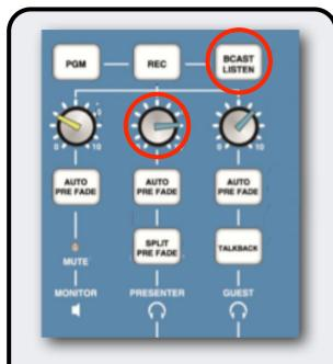
When you are ready to read. Press the *BCAST LISTEN* button to illuminate it and you will hear the station output.
